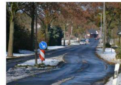
chicane-style traffic calming slows vehicles approaching village - north and south approaches
