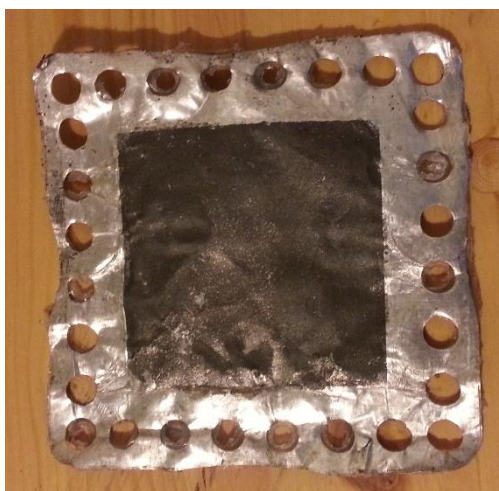
Figure 15: Aluminium electrode current collector coated with graphene nano platelets
