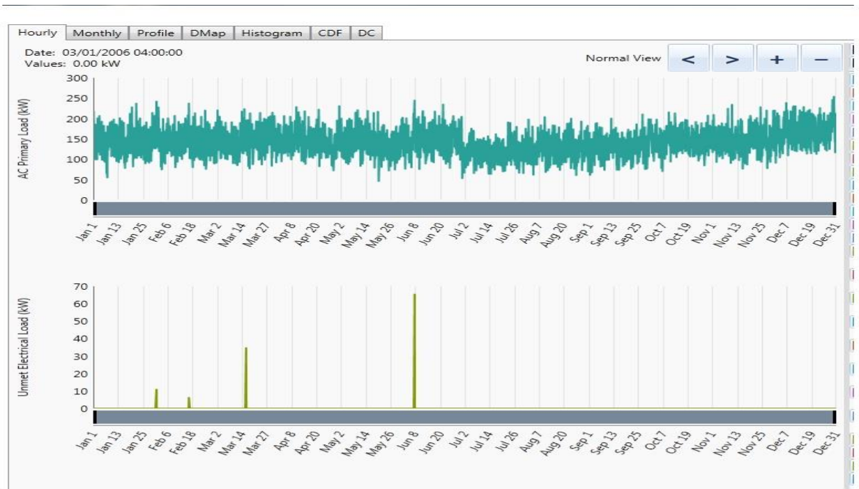
Figure 7: AC primary load profile (top) and capacity shortages (blackouts) (bottom) when hydro-diesel hybrid system is used for future demand
