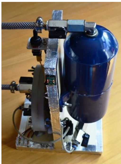
Figure 17 : Initial battery testing setup used for material and electrolyte stability testing
